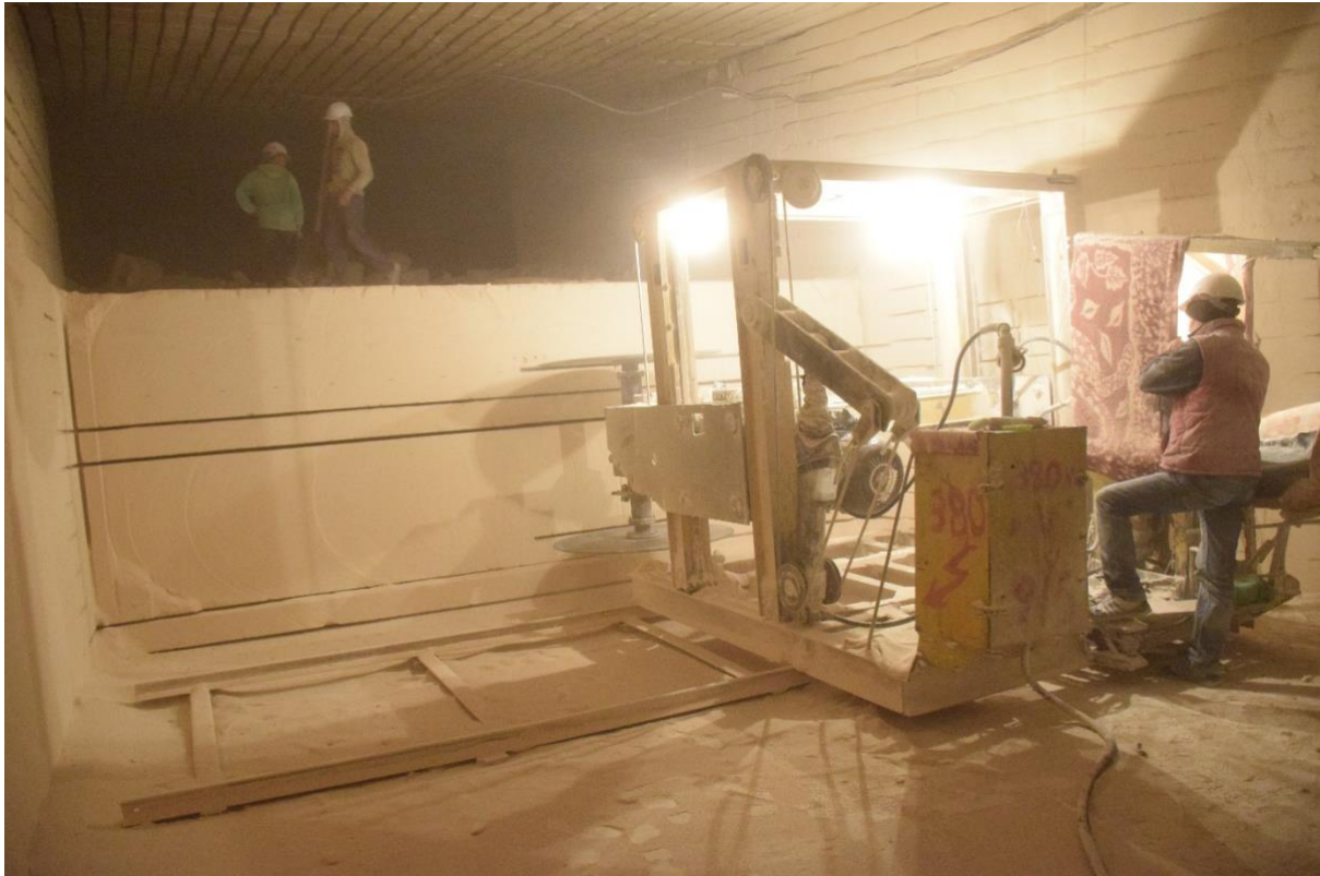
Picture 12 Limestone cutting at SOE Branesti mine
