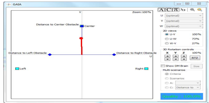
Fig. 6. Suggested direction for the wheelchair with 3 % increase in D_1 or 3 % decrease in D_r .
